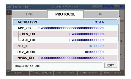
Fig 3.21 Parameters for OTAA (LoRaWAN V1.0)
