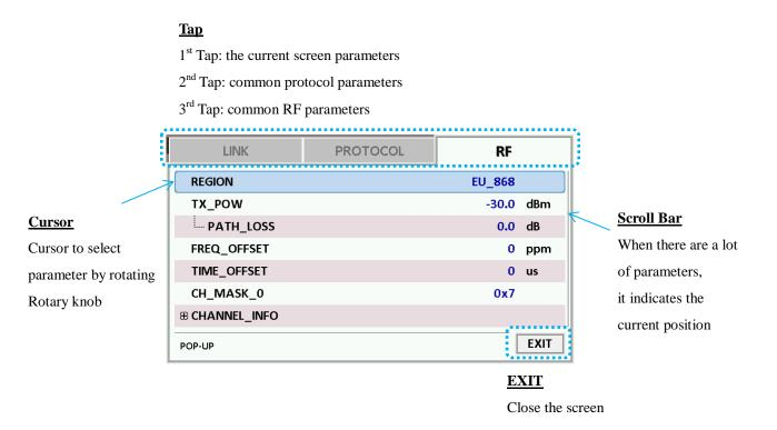
Fig 2.9 Parameter Configuration Screen
