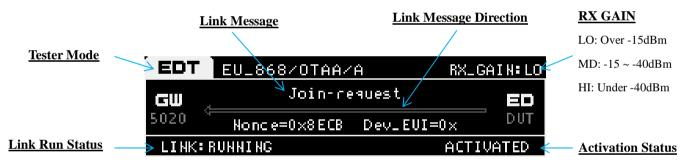
Fig A.4 RWC5020M Screen in running state
