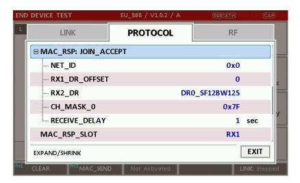
Fig 3.5 Parameters for Join-accept Message
